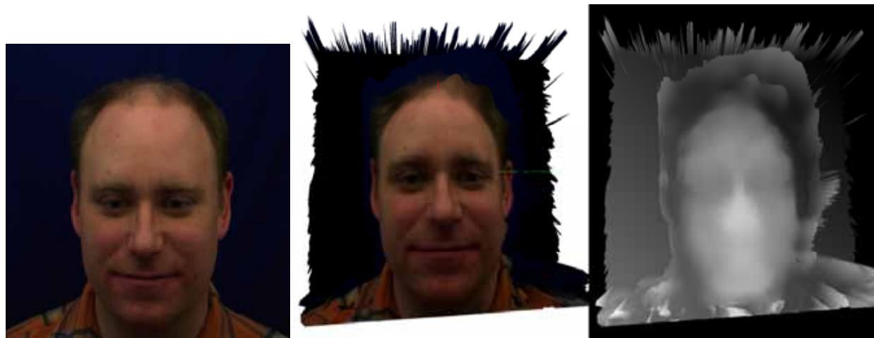
Patch sweeping result: original view (left), synthesized view (middle), depth map (right)
